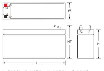
5.94 (151) **W**: 2.08 (53) **H**: 3.66 (93) HT: 3.89 (99) Tolerances are +/- 0.04 in. (+/- 1mm) and +/- 0.08 in. (+/- 2mm) for height dimensions.
